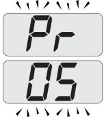
• Press keys 15 and 17 (Fig. 8.3) at the same time until the value of parameter 05(00=G20) is displayed on the LCD display (Fig. 8.6).
