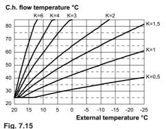
The K coefficients is a parameter that increases or reduces the boiler flow temperature when the outside temperature changes.
