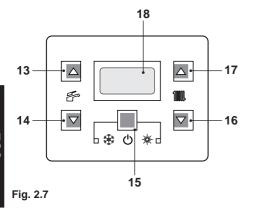
The LCD display displays the boiler temperature (primary circuit) and the  $rac{1}{2}$ ; symbol; the  $^{\circ}C$  symbol slowly flashes Fig. 2.8.
